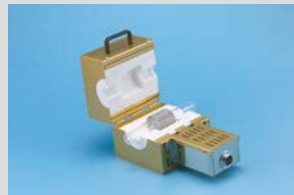
管状炉 Tube-shaped furnace
