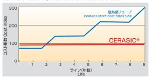
コスト指数:CERASIC製チューブの9年間での投資金額を100として算出 Cost index was calculated by regarding the investment cost of CERASIC® tube for 9 years as 100.
