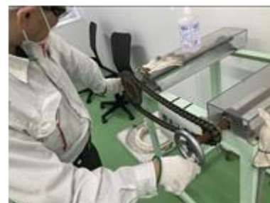
Risk of caught in machine (Kariya Facility)
